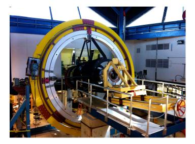
Figure 3: Telescope simulator at Fermilab. The purpose of this setup is to mechanically test the fully integrated camera, fiter and shutter jukebox and hexapod adjustors. Lenses are directly shipped to the telescope, so mock weights are used instead. Also the cryogenic system and the detector grounding are tested with this fixture.
