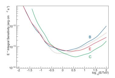
Figure 2: Integral sensitivity for candidate configurations B, C, and E, for point sources observed for 50 hours at a zenith angle of  $20^{\circ}$  [11].
