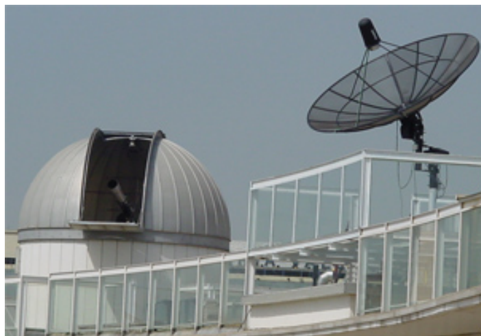
Figure 1: View of the Aula d'Astronomia with the 5 m dome, where the apochromatic 7'' telescope is seen beside the 3 m radiotelescope. Courtesy of Enric Marco.
