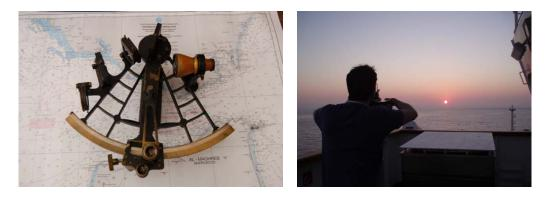
Figure 2: *Left*: Modern sextant for teaching astronomical navigation, in use at La Coruña University. *Right*: Measuring the solar azimuth with an alidade.
