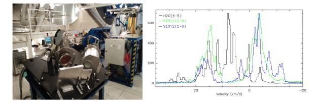
Figure 4: *Left*: Receivers installed at the Yebes 40-m radio telescope that allows the simultaneous observation of the frequency bands centered at 22 and 43 GHz. *Right*: example of obtained spectra.
