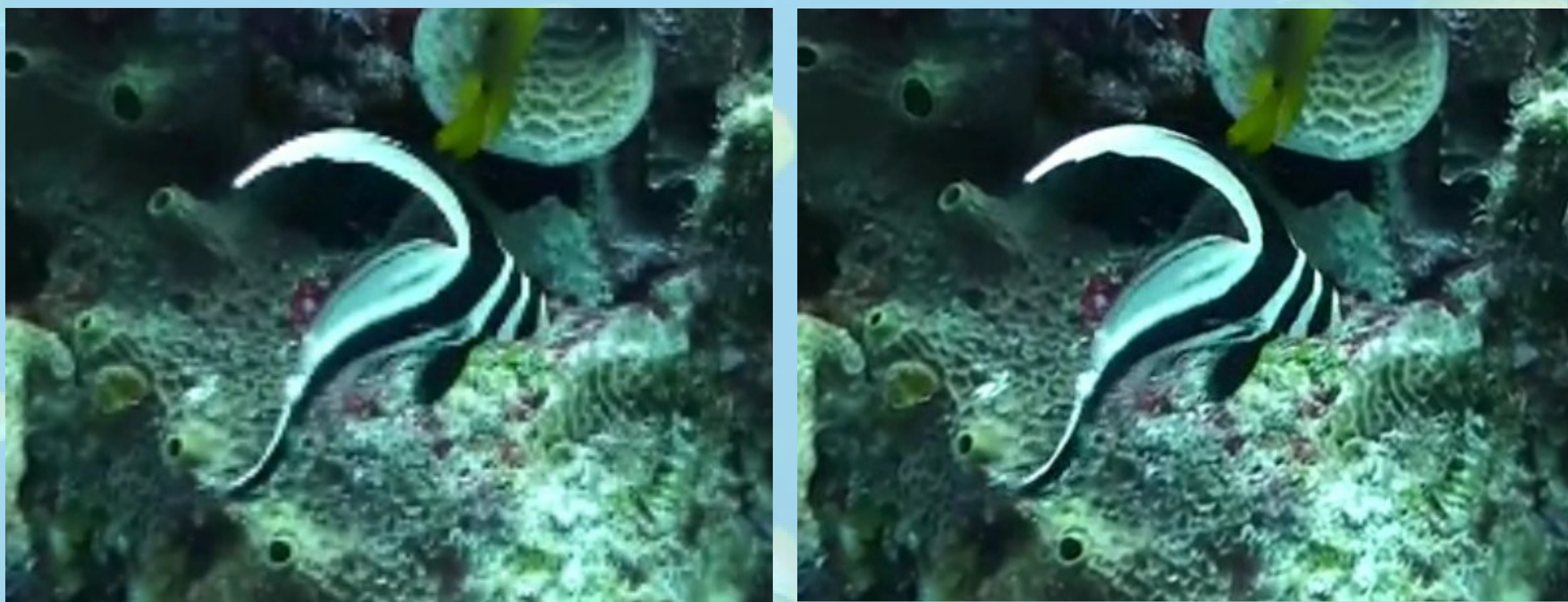
Fig.1: Frame extracted from a submarine video. Left: interpolation applied (showing pixelation). Right: MACABM Super Resolution method applied.
