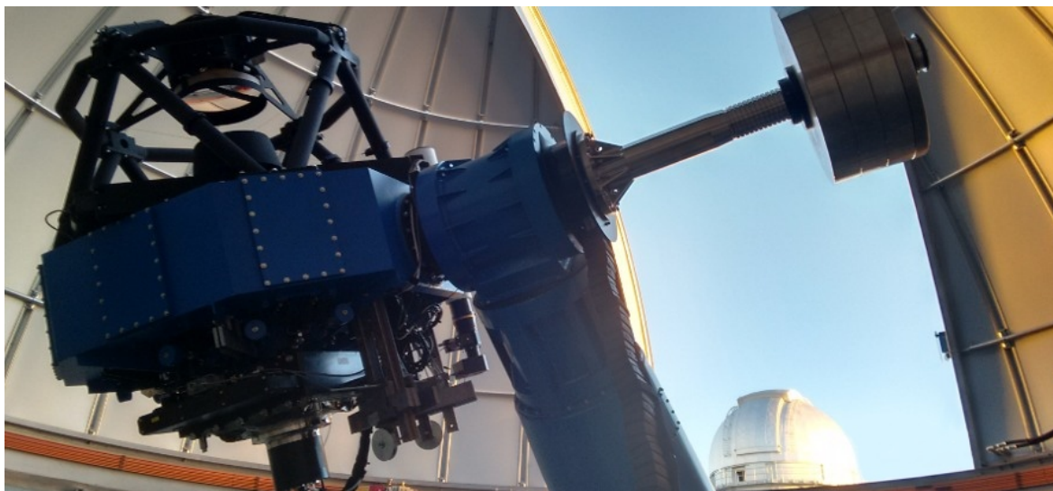
Figure 1: A picture of JAST/T80 with the dome open. The secondary mirror (on top) and the intermediate baffle are clearly seen. T80Cam, at the Cassegrain focus, is also seen. Out of the dome, JST/T250, the main telescope of the OAJ.
