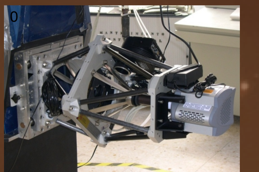
Figure 2. FastCam installed at TCS (OT) offering a plate scale of 40 mas/pixel and 30ms time resolution.
