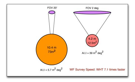
Figure 1: Survey efficiency of 10-m and 4-m telescopes compared. The speed at which one covers a given number of objects to a given S/N scales as the product of telescope collecting area A times viewing solid angle  $\omega$ . This product is 5.7 m<sup>2</sup> deg<sup>2</sup> for a 10-m telescope with a 20-arcmin FOV, and 39 m<sup>2</sup> deg<sup>2</sup> for a 4-m telescope with a 2-degree FOV. Survey speed is 7.1 times faster for the smaller telescope.
