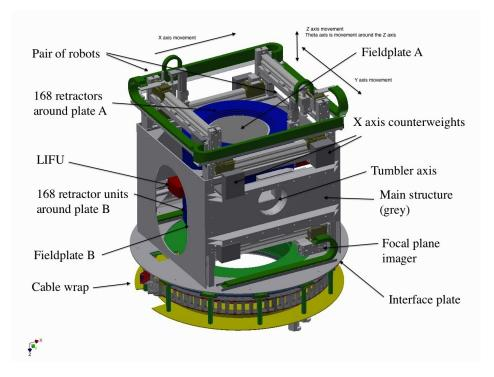
Figure 2: The final design of the WEAVE fibre positioner. Light from the primary mirror enters from below. Of the two field plates, plate A is shown in the configuration position and plate B (below) is in the observing position. A 180-degree rotation around the tumbler axis reverses their positions, while a 90-degree rotation places the large IFU (LIFU, red in the image) in the observing position. The two x-y robots are at the top. The blue drums are the fibre retractors.
