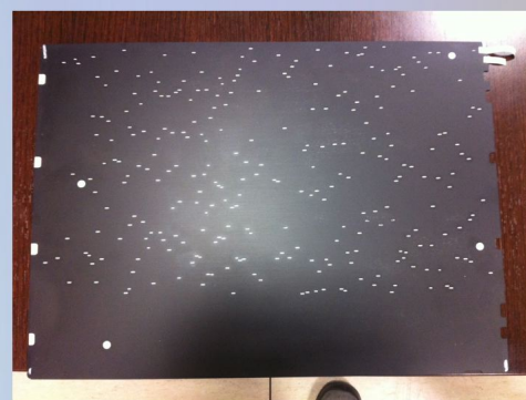
Image of the focal plane mask punched at the GTC workshop, courtesy of Antonio Cabrera. The round holes correspond to the fiducial stars used for plate positioning.
