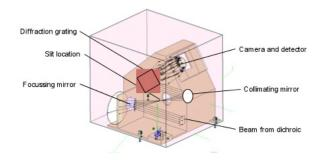
Figure 3: Near infrared channel (SWIR) module outline including its optical design and mechanical envelope (diagram courtesy of G. Ramos Zapata).
