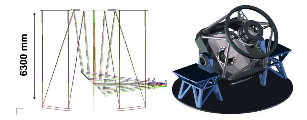
Figure 2: Left panel: Optical configuration for one of the HEXA design. In this case, a Richie Chretien Nasmyth configuration with a 1° field–of–view. Right panel: 3D model for the telescope and the two Nasmyth platforms.
