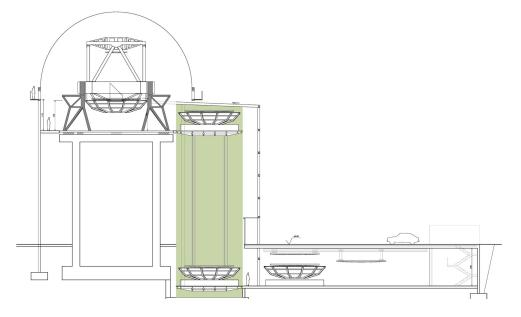
Figure 6: The Dome, the telescope and the service module.
