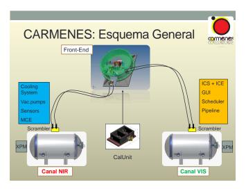
Figure 2: Layout of the instrument design. Two spectrographs (channels), one in the VIS and one in the NIR wavelength ranges will be thermo-mechanically stabilized in the 3.5 m telescope's Coude room and attached to the telescope with fibres through a front-end adaptor.
