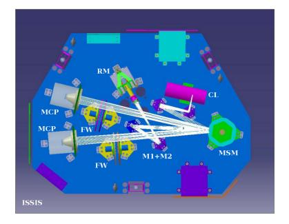
Figure 2: The optical bench assembly (without cover) for ISSIS.
