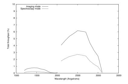
Figure 4: Throughput curves for the whole system in the two ISSIS channels. The estimate includes the two telescope mirrors, the ISSIS mirrors, the detector, and the grating (the latter one only in spectroscpy mode); filters are not considered.
