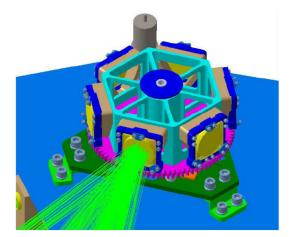
Figure 3: The mode selection mechanism (MSM) employed in ISSIS.
